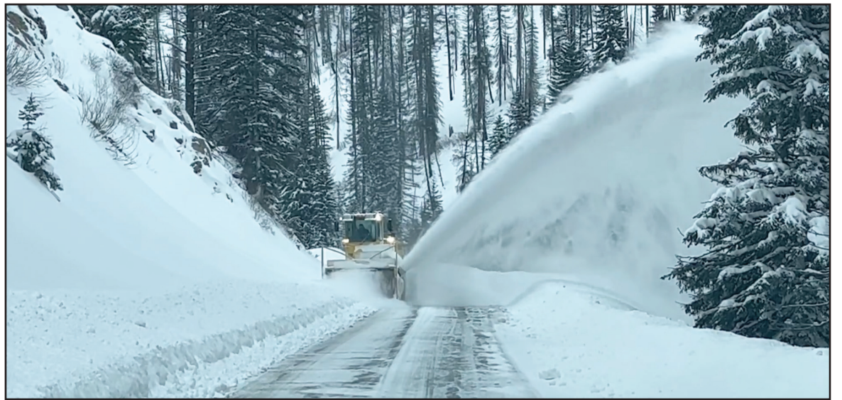
A rotary snowplow cleared Highway 21 on January 14th. Courtesy of Boise County Deputy Mackenzie
