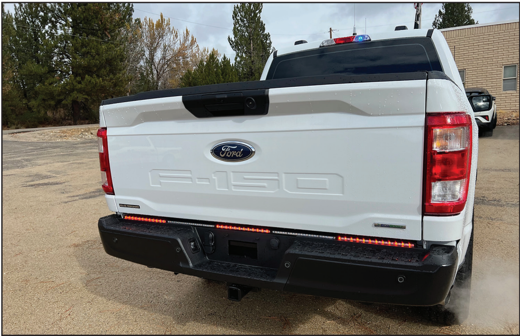
There are no longer lightbars on top, which are more expensive to install and become encrusted with snow in the winter, blocking the glow of the emergency lights. The lightbars are being phased out throughout Idaho and this county is one of the last to still have them, according to Boise County Deputy Reeder.
