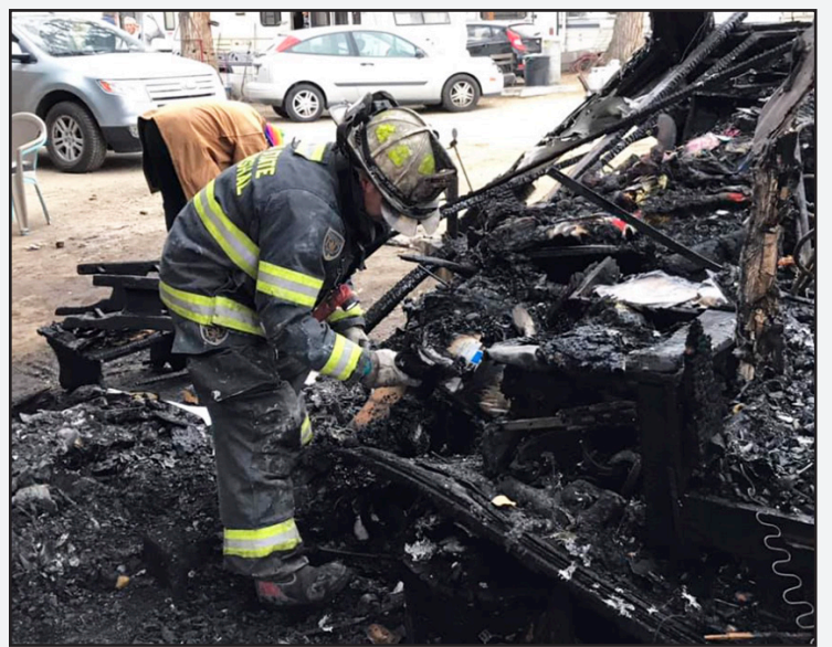
Courtesy of the Idaho State Fire Marshal's Office HORSESHOE BEND -- Deputy Alan Perry investigated a fire that occurred during the late evening hours on Monday in Horseshoe Bend. Although Horseshoe Bend Fire was able to extinguish the fire quickly, the RV being used as a permanent residence was a complete loss. The cause was determined to be an overloaded electrical system due to several electric space heaters being used. The Red Cross is assisting the couple with their immediate needs.
