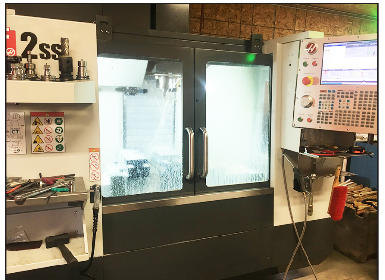
This is their newest 2018 machine that takes in computer coordinates to make and design metal pieces for assembly.
