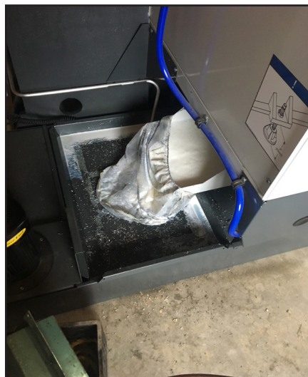
Metal filings are filtered out in this closed system that recycles the lubricant and water.
