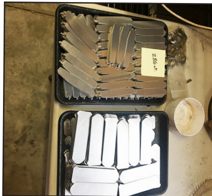
Metal is bought in thick sheet, cut into appropriate sizes and used to fabricate knife parts with the use of several machines.
