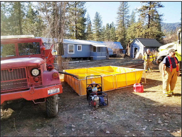
We set up a 2500-gallon fold-a-tank to ensure there was more than enough water on-hand, to make certain the fire stayed where it belonged. There was at least 10,000 gallons of water on-hand. — with Steve Moore and Sam Pecorito at Frenchman's Flat.
